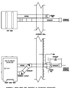
SIDEWALL VENT WITH TEE (INTAKE) & COUPLING (EXHAUST)
